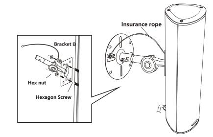
3 As shown in the following figure, bracket part A is fixed on the wall where the speakers need to be installed (the screws of the fixed bracket assembly A are owned).
