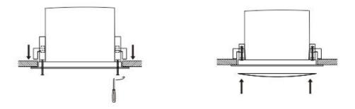
4. Finally, check whether the speaker is installed in a firm and reliable way.
