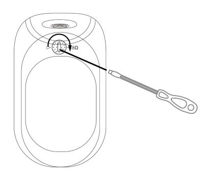
Use A Flat-Blade Screwdriver to align the holes to adjust: General amplifier turn to 80hm button / Turn to the specified button to connect with constant voltage power amplifier.
