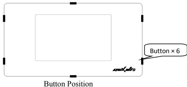
Open the middle button with thumb or other objects (not sharp) slide from upper left corner gap to right, open the rest buttons by slide along the gap. You will hear a sound like 'Click' when each button is opened.
