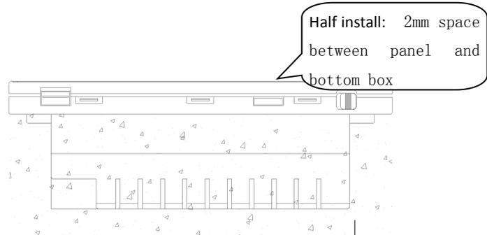
⑦ Fastening the panel after test is ok and
