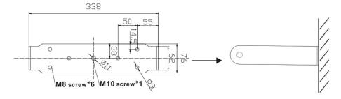
2. Remove the screws on the horn box for spare use and remove the waterproof seal cover. Connect with the wiring diagram according to the customer's needs, and tighten the seal cover after connection.
