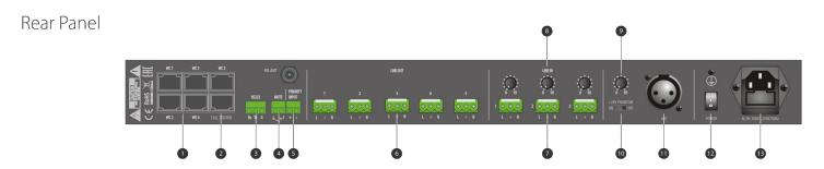
1. Connectors for MAG505S wall control | 2. Connector for MAG505R page station | 3. RS232 serial interface | 4. External mute | 5. Priority audio input | 6. Stereo audio outputs | 7. Stereo audio inputs | 8. Inputs gain control | 9. Microphone gain control | 10. Phantom power switch | 11. Microphone input | 12. Power switch | 13. Main power connector
