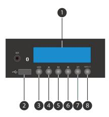
1. LCD screen | 2. USB slot | 3. Mode button | 4. Backward / Set FM frequency and preset | 5. Play-pause / Radio frequency scanning mode 6. Forward / Set FM frequency and preset | 7. Repeat button / Save FM preset | 8. Mute - power button / Exit
