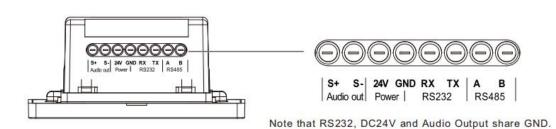
From Left to Right: Audio Output S+ Audio Output S DC24V Input GND RS232-RX RS232-TX
