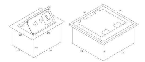
As is shown in the picture above, on the left is the dimension of D6272. Ground installation depth is at least 132mm. On the right is the dimension od D6272B. Ground installation depth is at least 72 (66+6) mm.
