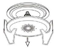
Step 3: Press the open hole in advance, install the product to the ceiling, and lock the screws.
