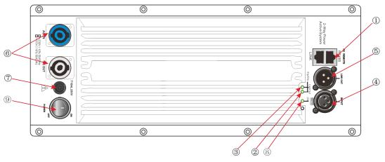
(1) Control Interface: Connected to the computer through RS485, and a RS232-USB interface is required for conversion.
