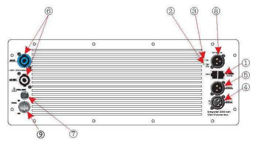
(1) Control Interface: Connected to the computer through RS485, and a RS232-USB interface is required for conversion.
