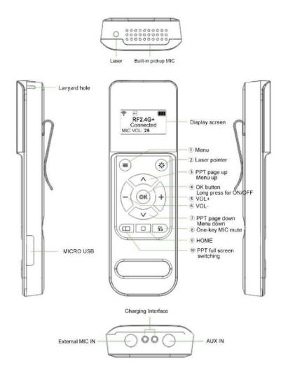
① "≡" Main Menu Button Press this button to enter the main menu interface where "PPT Settings", "Reverb Settings" and "System Settings" are displayed.
