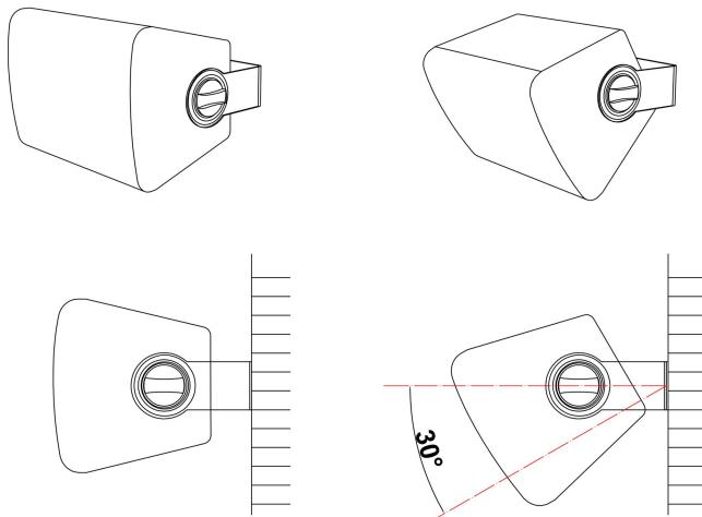
Select an appropriate position on the facade to install two screws for the column speaker. Attach the bracket as shown in the diagram and secure the speaker. If necessary, adjust the angle of the bracket to position the speaker up or down.
