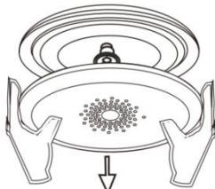
Step 4: After the product is fixed, reload the mesh mask.
